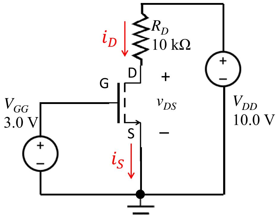
Known: NMOS,  $V_{TO} = 1.0$  V,  $\lambda = 0$ ,  $K'_n = 25\mu\text{A}/\text{V}^2$ ,  $\frac{W}{L} = 10$
