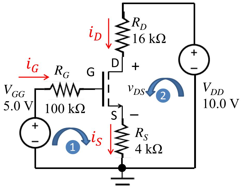
Known: NMOS,  $V_{TO} = 1.0 \text{ V}$ ,  $\lambda = 0$ ,  $K'_n = 25 \mu\text{A}/\text{V}^2$ ,  $\frac{W}{L} = 10$
