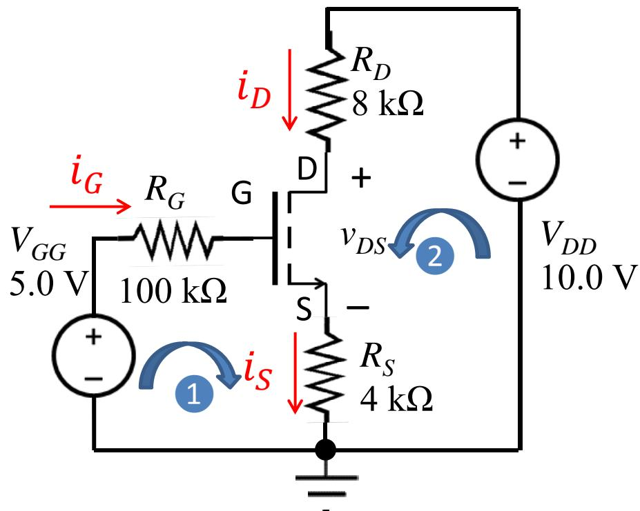
Known: NMOS,  $V_{TO} = 1.0 \text{ V}$ ,  $\lambda = 0$ ,  $K'_n = 25 \mu\text{A}/\text{V}^2$ ,  $\frac{W}{L} = 10$
